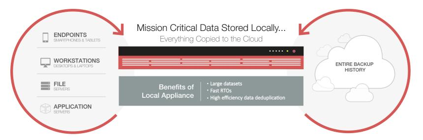
Since your most critical data is within your most recent backup, it's safe to assume that most recoveries would come directly from the hybrid appliance. With the hybrid appliance being local, data recoveries happen over LAN speeds instead of across slow WAN connections to the cloud provider.
